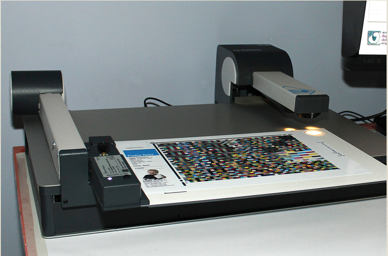
The Barbieri Spectro LFP is for flatbed spectrophotometry and is capable of both reflective and transmissive measurements.
